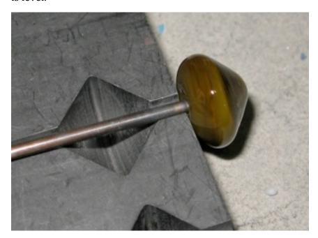
6. You also want to make sure that you have a pointier bottom. I'm going to add some frit so that will be enough to get a nice tip. At this point, when I know the glass is hard, I test the top being very careful not to have it land in my lap. Spins okay so it is back into the flame for a little heat and then into the kiln.
