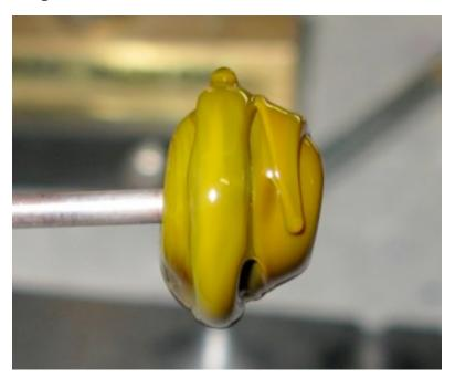
4. Start to shape in the larger cavity. This is the tricky part. You want to push the soft glass into the end of the bead roller without pushing the mandrel through. To get a good pointy end, you need to give a decent amount of pressure. Check to make sure that you haven't pushed the mandrel through. At this point but you have your basic shape so you can heat the bead and as you put it into the cavity, you can pull the mandrel to your right (provided you are right handed)
