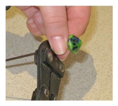
Notice the uneven mandrel from making the cut? I sand the mandrel smooth with my Dremel sanding disc. I hand sand the shaft of the mandrel with 180 grit sandpaper and then buff until I'm happy.
