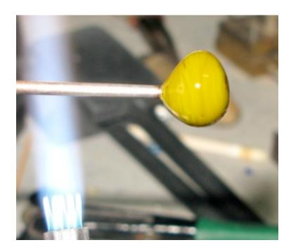
2. Using your stubby bi cone bead roller, start to shape on the  $2^{nd}$  smallest cavity making sure that you don't push the mandrel too far to the bottom. If you do this, simply reheat the glass and let gravity pull it down and then repeat the shaping.
