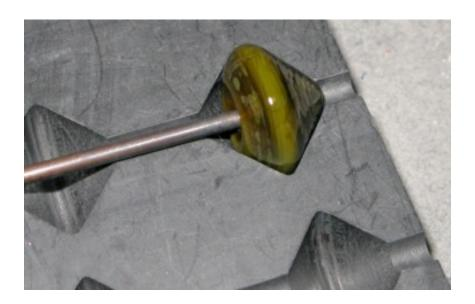
5. To get a nicely shaped even top, use the edge of the bead roller to make sure it is level.
