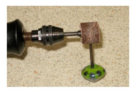
A good spinning top should last nearly 45 seconds and the mandrel should remain perpendicular until it starts to slow down. If you don't have a sharp enough point on the bottom of your top (oxymoron, I know), your mandrel is going to spin like it's bent and will not last long. (notice the shadows cast by the white top's mandrel)
